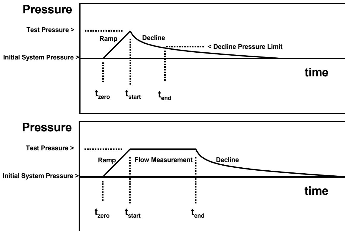
**Figure 2.3.2** Typical pressure / time traces for pressure-based tests
