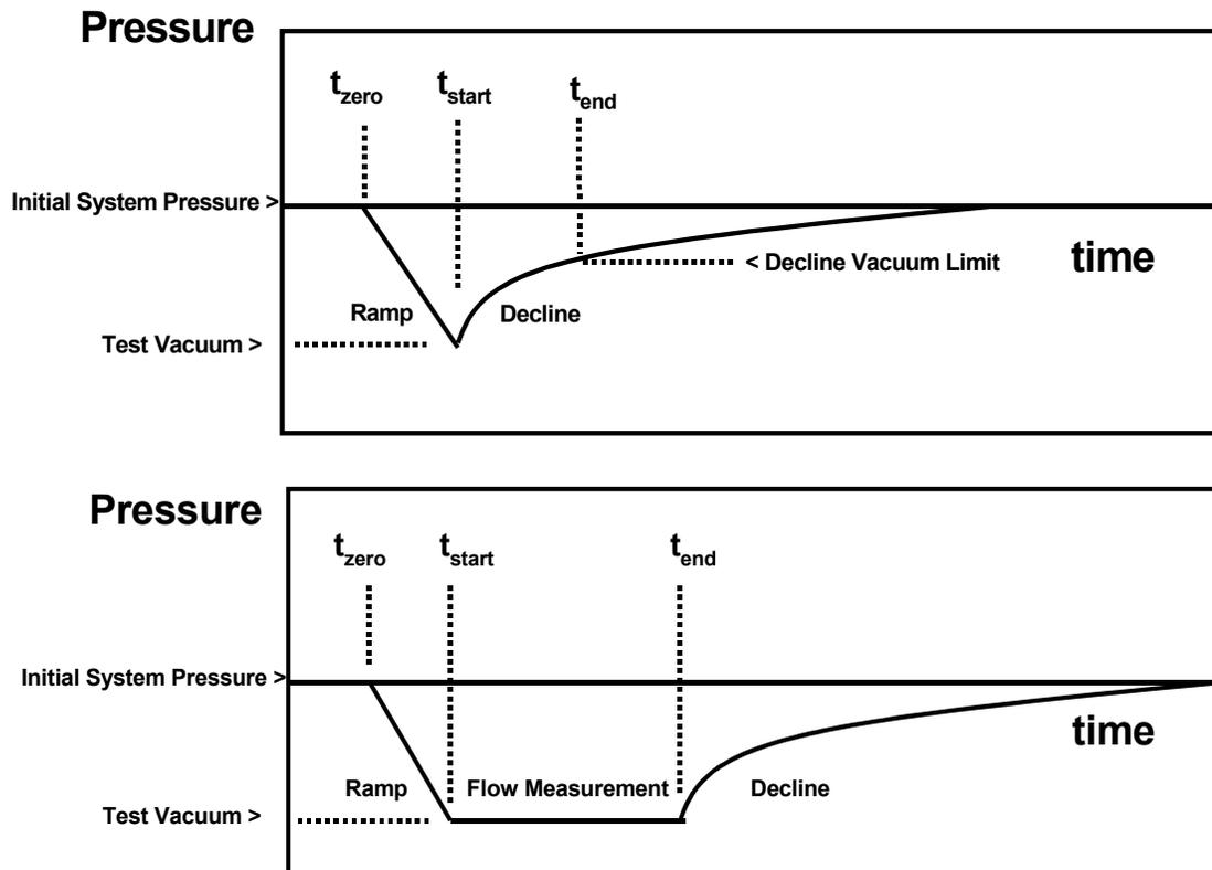
**Figure 2.3.1** Typical pressure / time traces for vacuum-based tests
