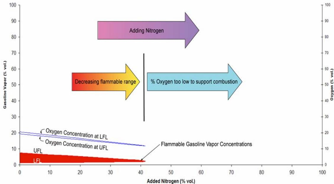
**Figure 1.** Flammable range for Gasoline/Air/Nitrogen mixtures. When more than 43% of the mixture is added nitrogen, the oxygen content is below 11% and no flammable mixture can form.
